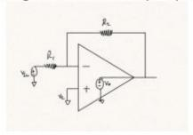
Let the negative input terminal be  $V_{INN}$ . We can express the output of the op-amp as  $-V_{INN}A_V$  or, equivalently, can express  $V_{INN}$  as  $-\frac{V_{OUT}}{A}$ . If we choose the second option, we can solve as normal:
